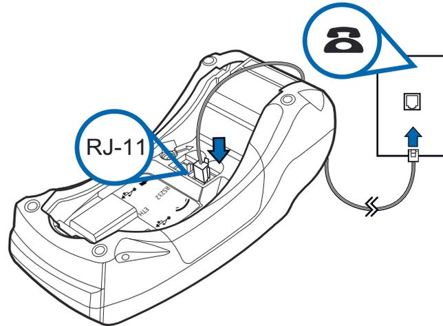
Figure 8 VX 520 Direct Telephone Connection
