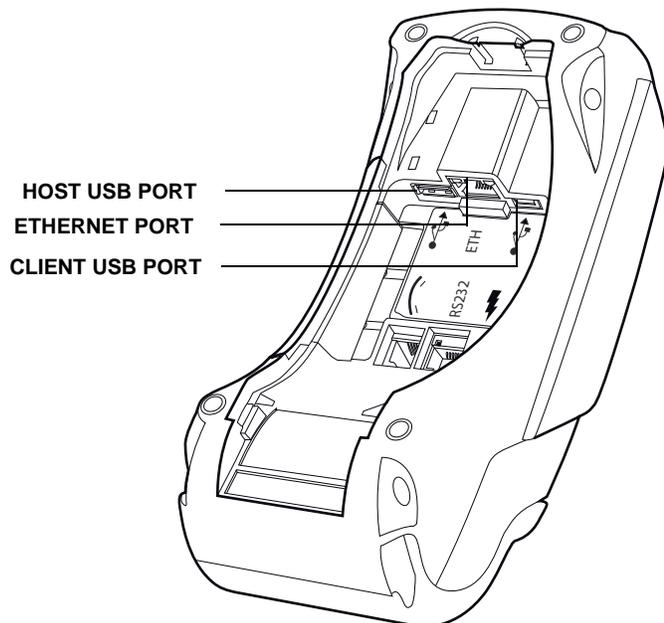
**Figure 5** Additional VX 520 Connection Ports
