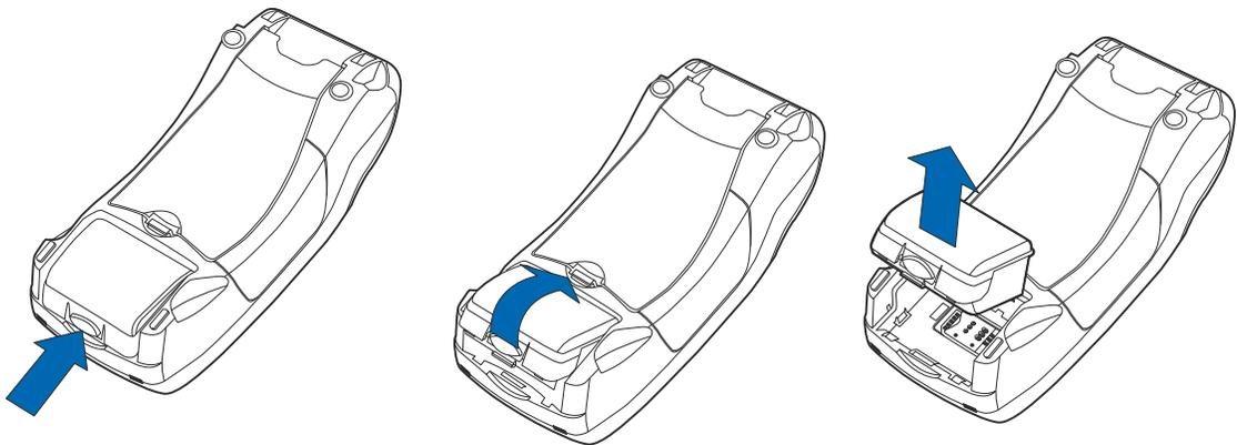
**Figure 7** Removing the Smart Battery
