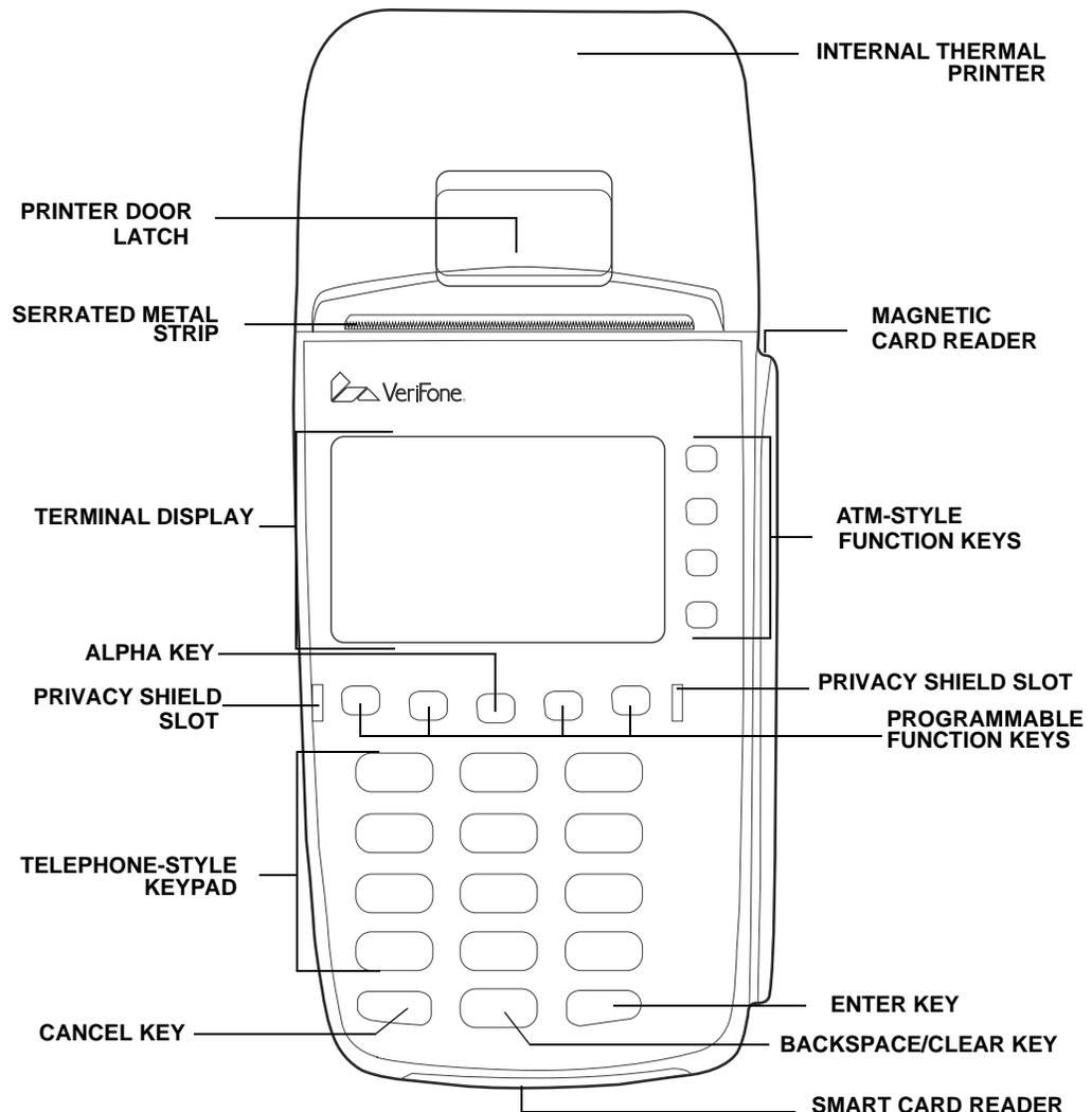
**Figure 2** VX 520 Terminal Features (Front Panel)
