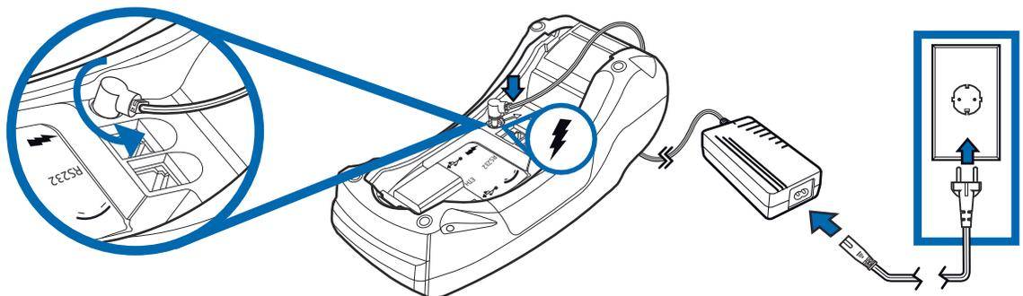
**Figure 19 VX 520 Power Pack Connection**
