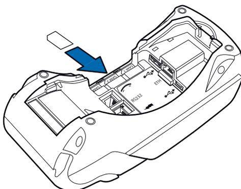
**Figure 14 Installing an MSAM Card**
