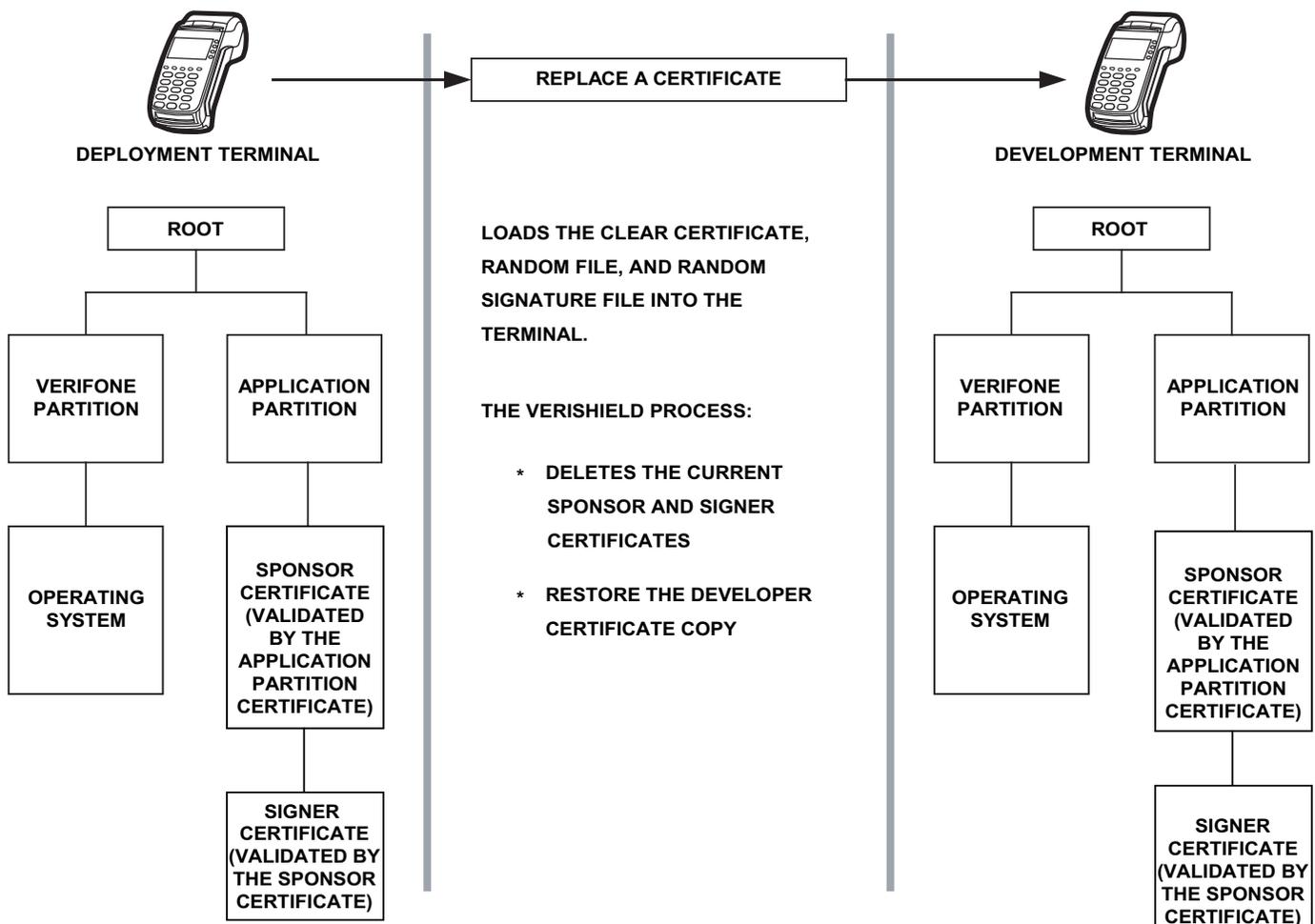
**Figure 31 Certificate Replacement Process**
