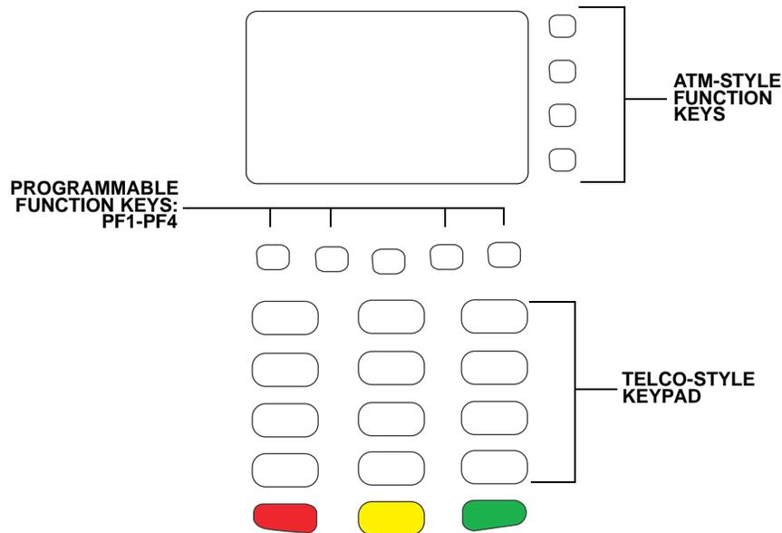
Figure 23 Front Panel Key Arrangement
