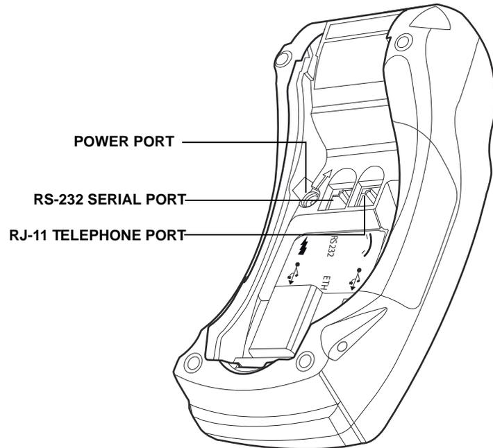
**Figure 4** VX 520 Power and Connection Ports
