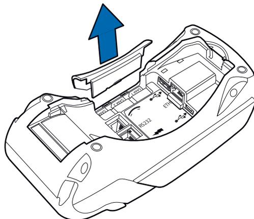
**Figure 13 Removing MSAM Cover**
