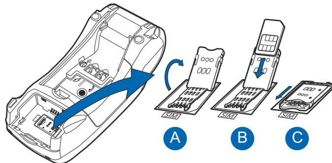
**Figure 16** Inserting SIM Card
