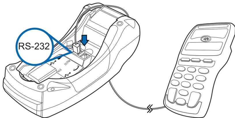
**Figure 17** VX 520 Sample PIN Pad Connection
