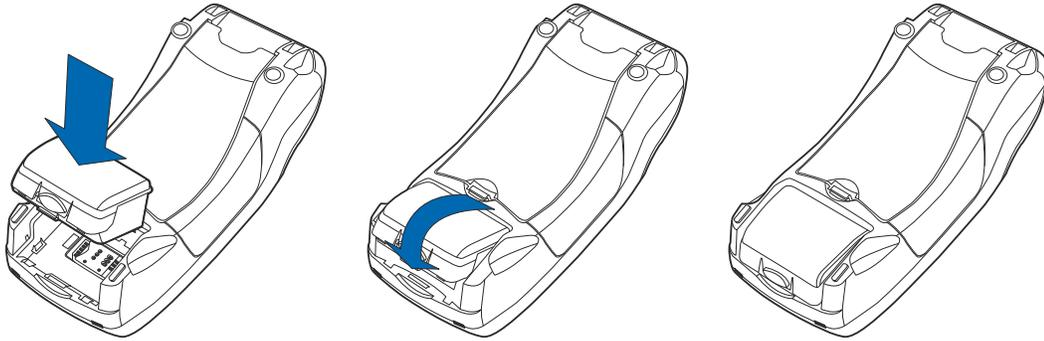
**Figure 6** Installing the Smart Battery
