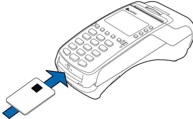
Figure 21 Inserting a Smart Card
