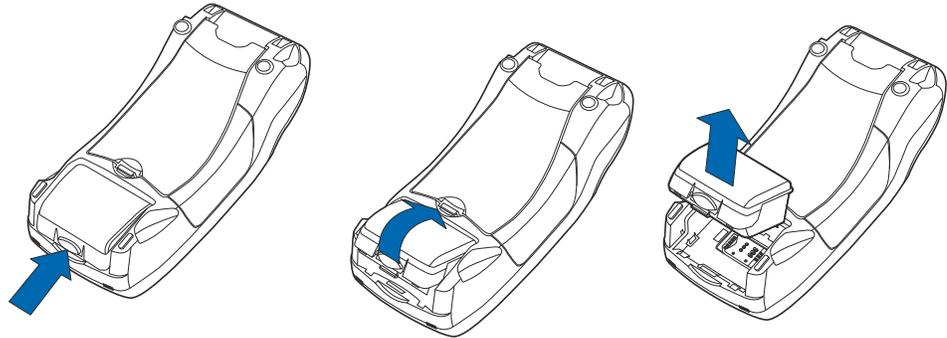
**Figure 15** Removing the Smart Battery
