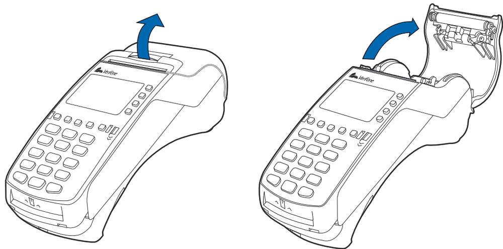
**Figure 9** Opening the Printer Cover
