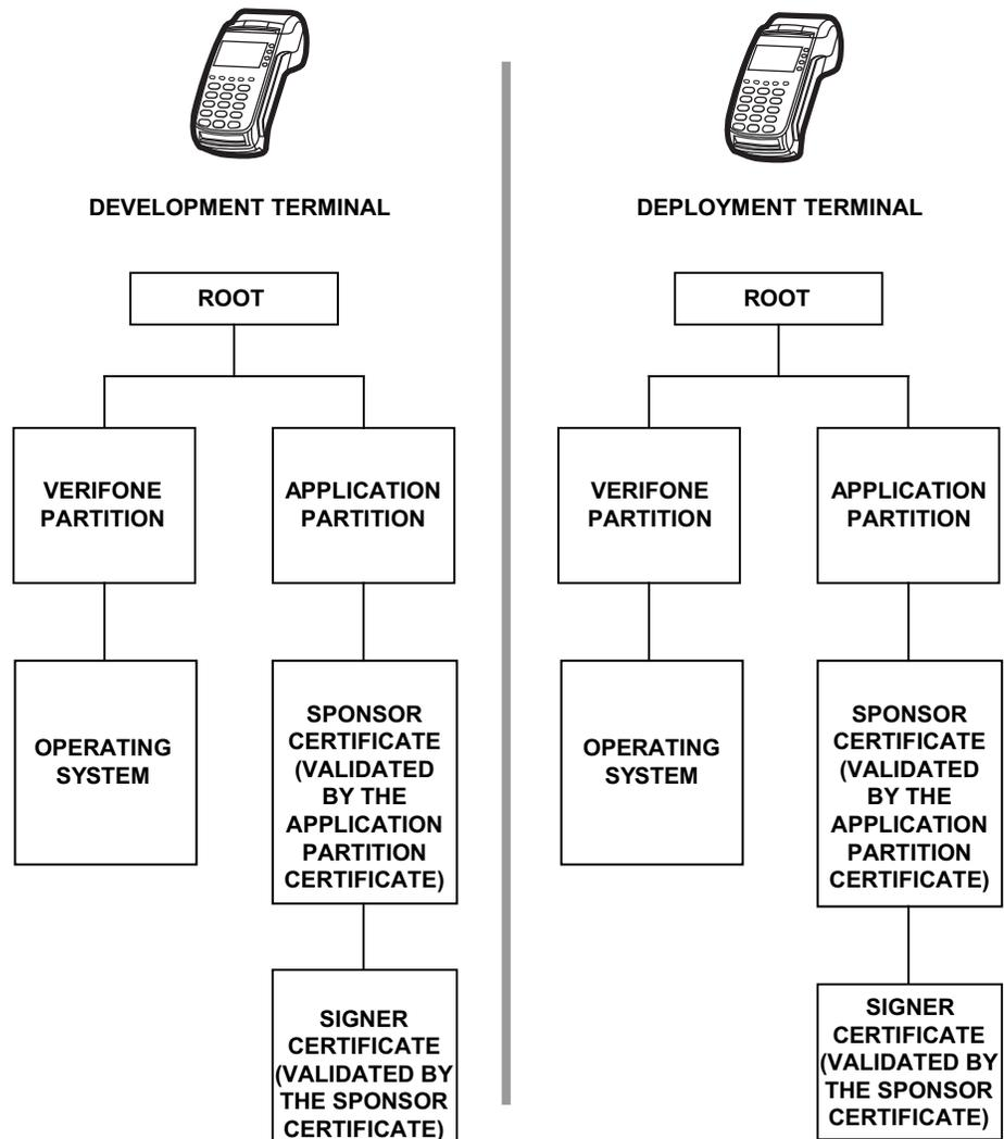
Figure 30 Certificate Trees in Development and Deployment Terminals
